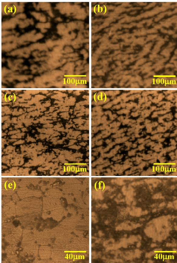
**Fig. 7.** Optical micrograph of 75% cold rolled Al-6Mg alloys aged at 300 °C for one hour (a) 0.0Sc, (b) 0.2Sc, (c) 0.4Sc, (d) 0.6Sc and aged at 400 °C for one hour (e) 0.0Sc, (f) 0.6Sc.
