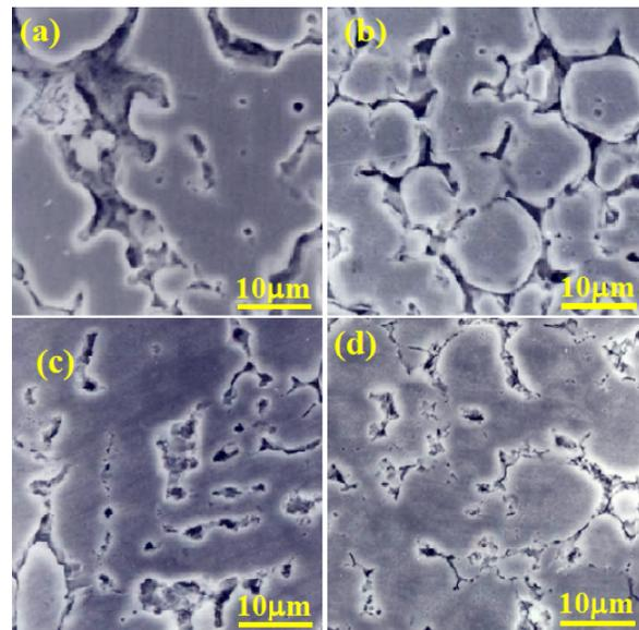
**Fig. 8.** SEM micrograph of cast Al-6Mg alloy (a) 0.0Sc (b) 0.6Sc and aged at 300 °C for one hour (c) 0.0Sc (d) 0.6Sc.
