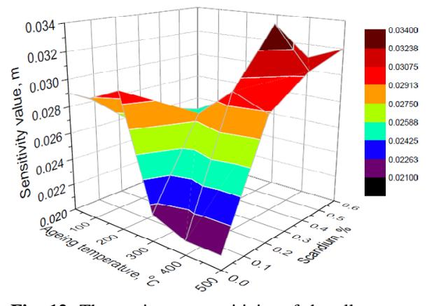
**Fig. 12.** The strain rate sensitivity of the alloys as a function of scandium content and ageing temperature.
