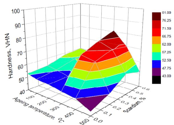
**Fig. 2.** The influence of scandium content and ageing temperature on the hardness of cast Al-6Mg alloys.
