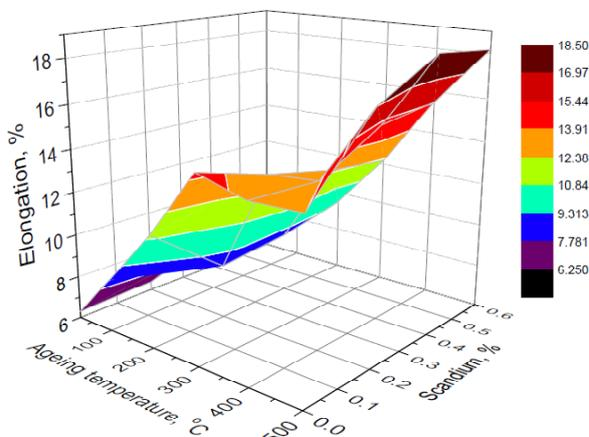
**Fig. 10.** The influence of scandium content and ageing temperature on the elongation of the alloys.
