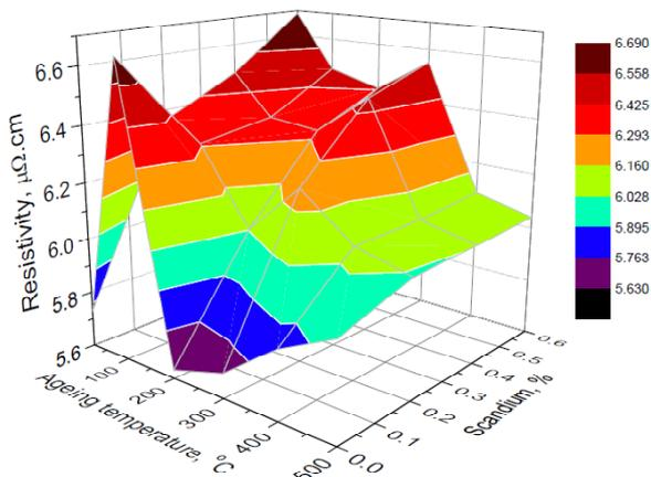
**Fig. 4.** The influence of scandium content and ageing temperature on the resistivity of 75% cold rolled Al-6Mg alloys.
