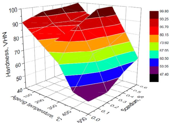
**Fig. 3.** The influence of scandium content and ageing temperature on the hardness of 75% cold rolled Al-6Mg alloys.
