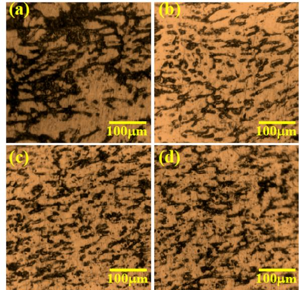
**Fig. 6.** Optical micrograph of 75% cold rolled Al-6Mg alloys (a) 0.0Sc, (b) 0.2Sc, (c) 0.4Sc, and (d) 0.6Sc.
