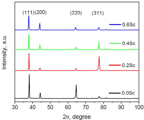
**Fig. 15.** XRD pattern for Al-6Mg alloys with different scandium contents.
