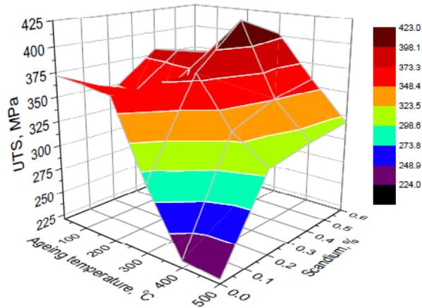
**Fig. 9.** The influence of scandium content and ageing temperature on the ultimate tensile strength of the alloys.
