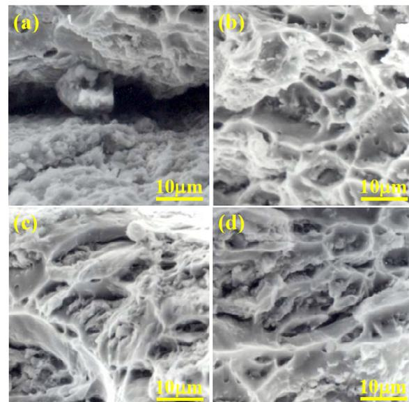
**Fig. 13.** SEM fractograph of 75% cold deformed Al-6Mg alloys aged at 300 °C for 1 hour (a) 0.0Sc, (b) 0.2Sc, (c) 0.4Sc, and (d) 0.6Sc after tensile tested at strain rate of  $10^{-3}\text{s}^{-1}$ .
