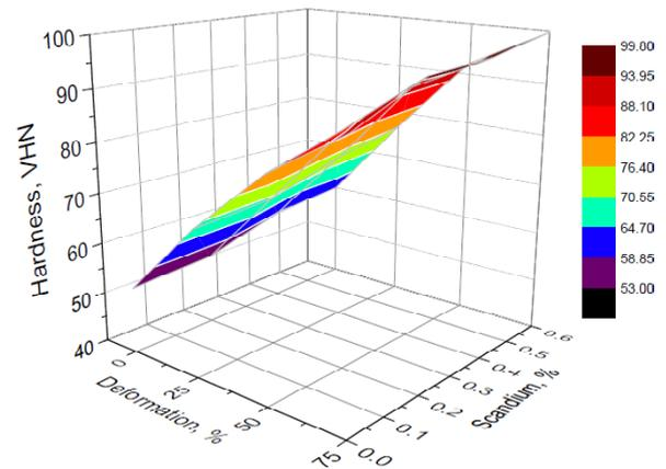
**Fig. 1.** The influence of scandium content and degree of deformation on the hardness of Al-6Mg alloys.
