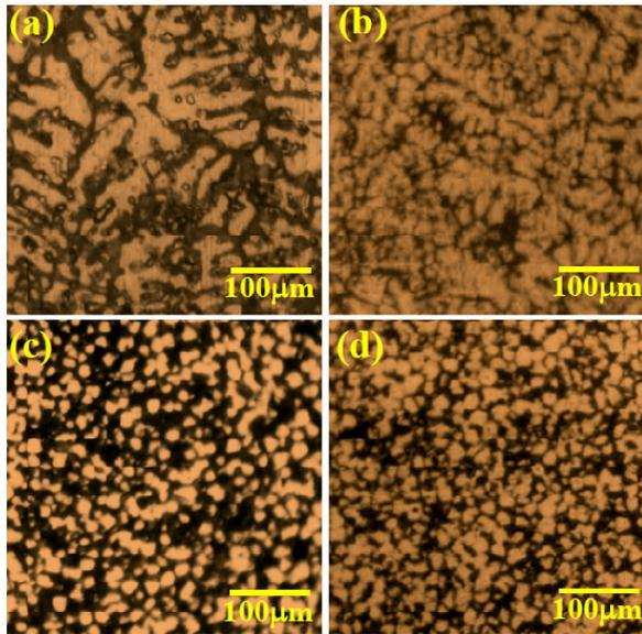
**Fig. 5.** Optical micrograph of cast Al-6Mg alloys (a) 0.0Sc, (b) 0.2Sc, (c) 0.4Sc, and (d) 0.6Sc.
