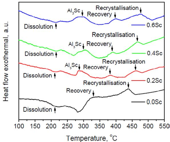
**Fig. 14.** DSC heating curve of Al-6Mg alloys with different scandium contents.
