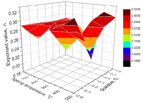
**Fig. 11.** The strain hardening exponent of the alloys as a function of scandium content and ageing temperature.
